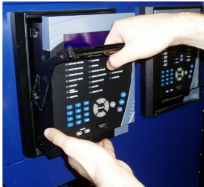
FIGURE 3-9: Slide Unit out of Case
