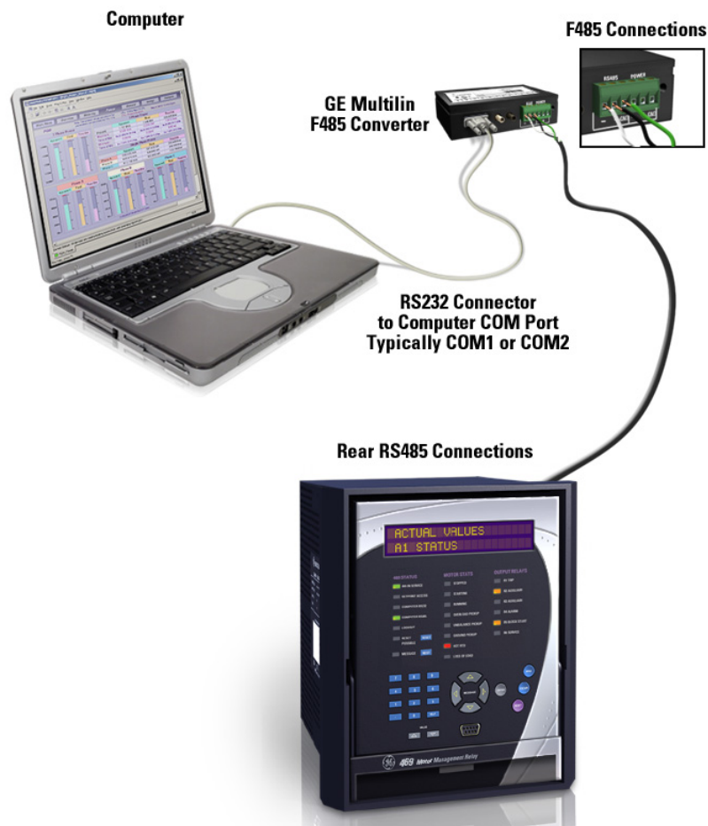
FIGURE 4-3: Communications using Rear RS485 Port
