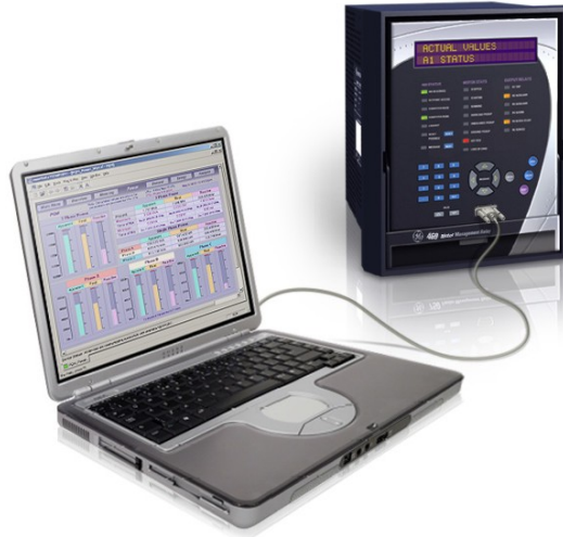
FIGURE 4-2: Communications using The Front RS232 Port
