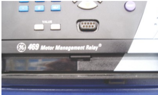
FIGURE 3-2: Seal on Drawout Unit
