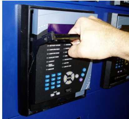
FIGURE 3-8: Rotate Handle to Stop Position
