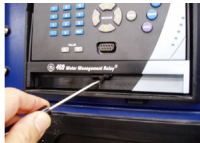
FIGURE 3-7: Press Latch to Disengage Handle
