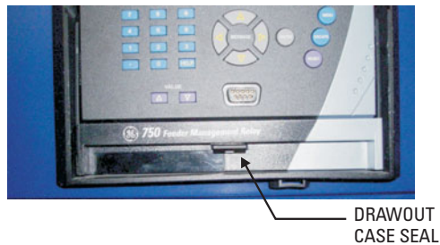
FIGURE 3-2: Drawout Case Seal
