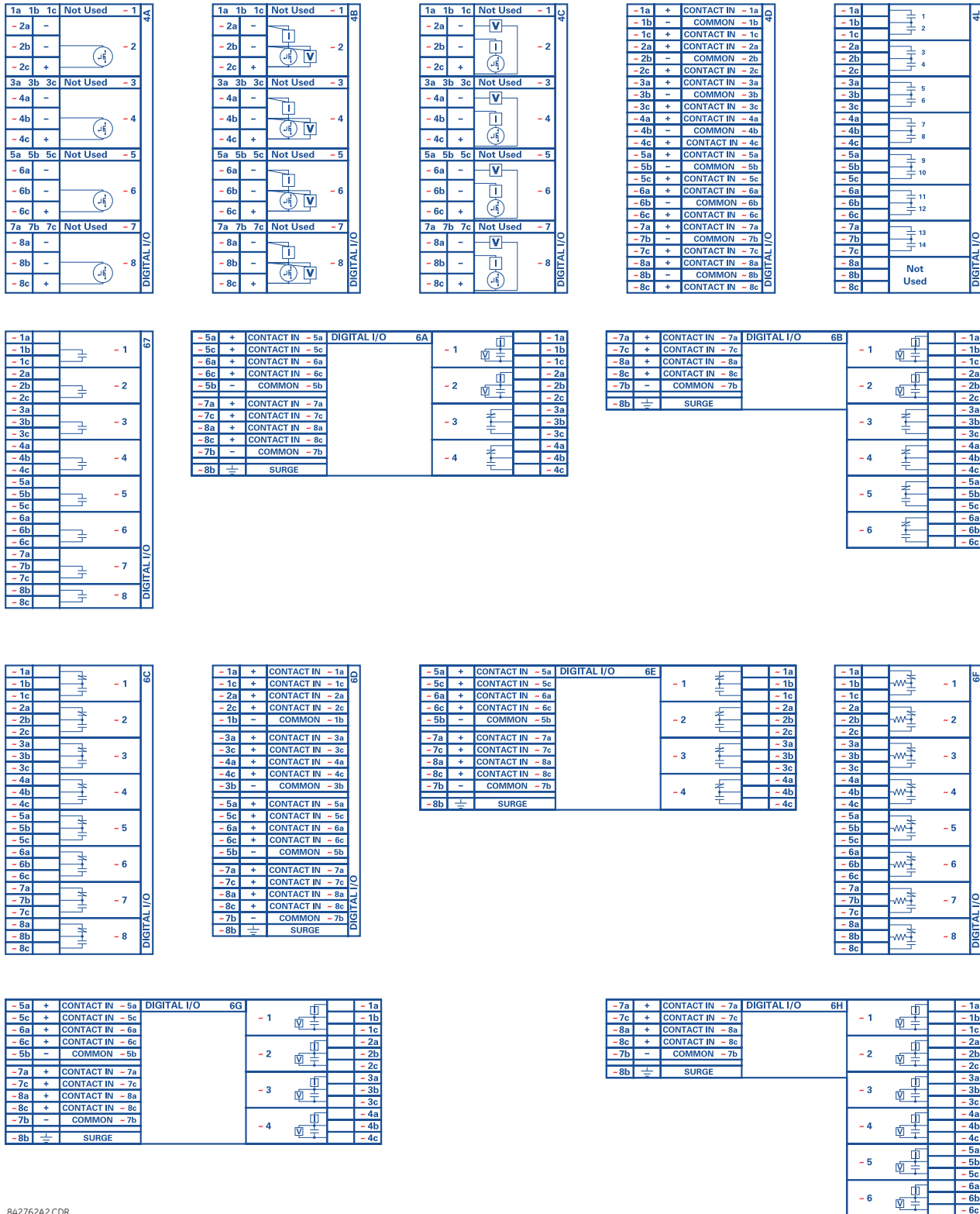
Figure 3-17: CONTACT INPUT AND OUTPUT MODULE WIRING (1 of 2)
